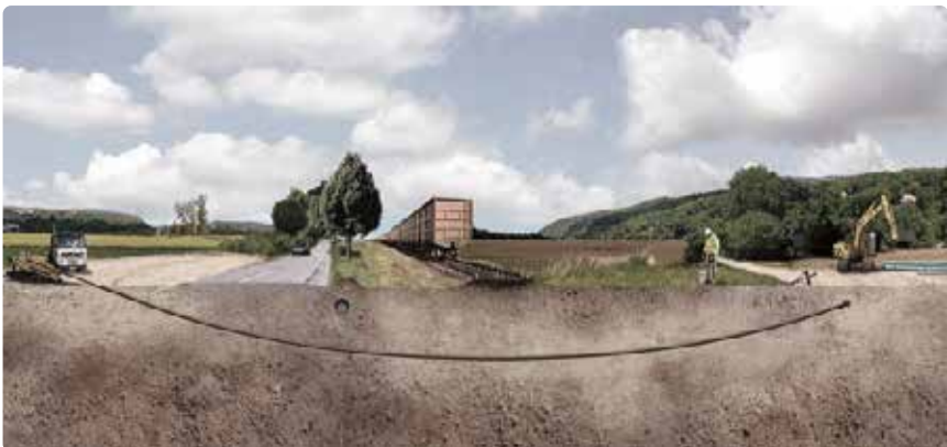
Schematic of horizontal directional drilling (HDD)
